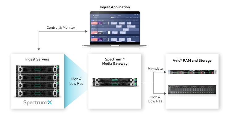
Spectrum Media Gateway provides a simple, low-cost solution to re-wrap MXF OP1a files to the MXF OPAtom format used by Avid's PAM and storage systems. MXF OP1a files ingested on Harmonic's Spectrum video server are automatically transferred to the Media Gateway, re-wrapped and transferred to the Avid system. The Spectrum Media Studio Ingest application can be used to control and monitor ingest operations on the Spectrum server and exchange metadata with the Avid PAM system.
